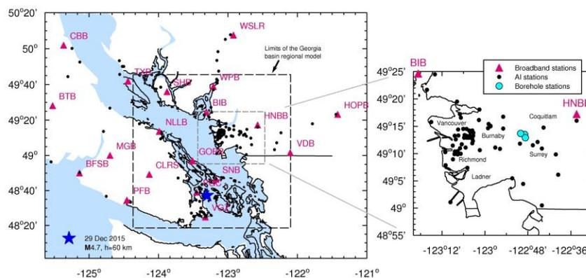
Figure 1. Overview map showing locations of CNSN and IA stations in relation to the Georgia basin velocity model limits (black dashed box) and Greater Vancouver (grey dashed box).
