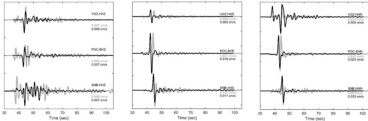
Figure 6. Comparison of empirical  $M$  4.7 earthquake recordings (gray lines) and synthetic (black lines) velocity time-series for the 3 closest broadband stations.
