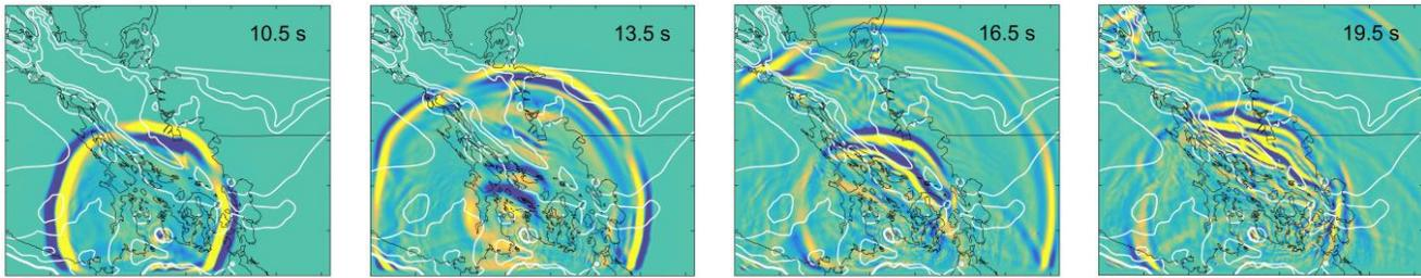
Figure 9. Time-snapshots of simulated ver. motion. Thin white lines are contours of basin  $V_P$  model structure at 500 m depth.
