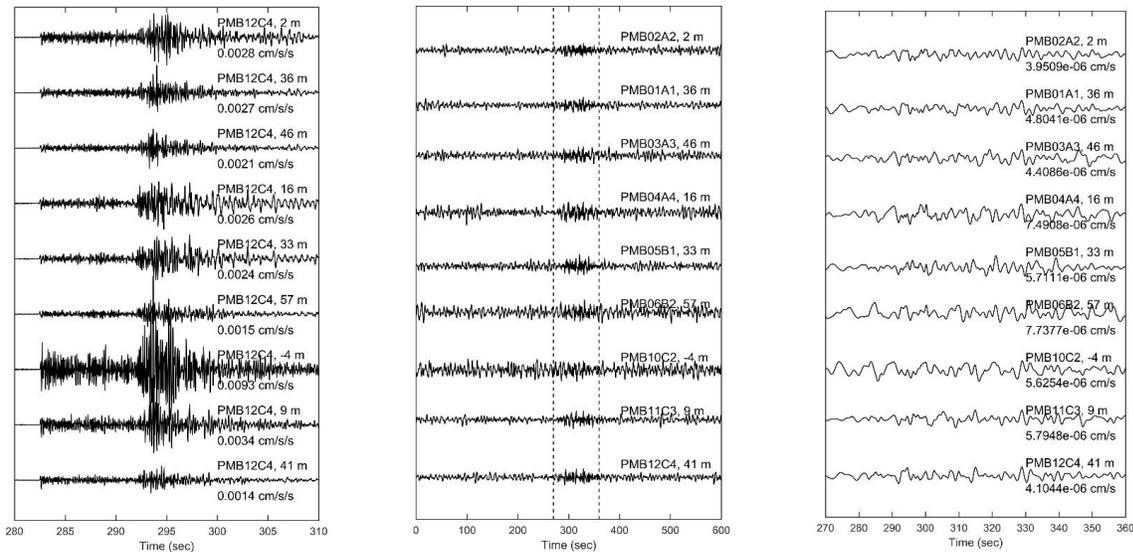
Figure 4. Vertical-comp. acceleration (left) and velocity time-series (middle) from IA stations are band-pass filtered with corners of 0.1 & 0.5 Hz. The right panel shows zoomed-in window (depicted with dashed lines in the middle panel). The name of stations, their depth of recordings, and peak ground velocity (PGV) values are reported on each trace.
