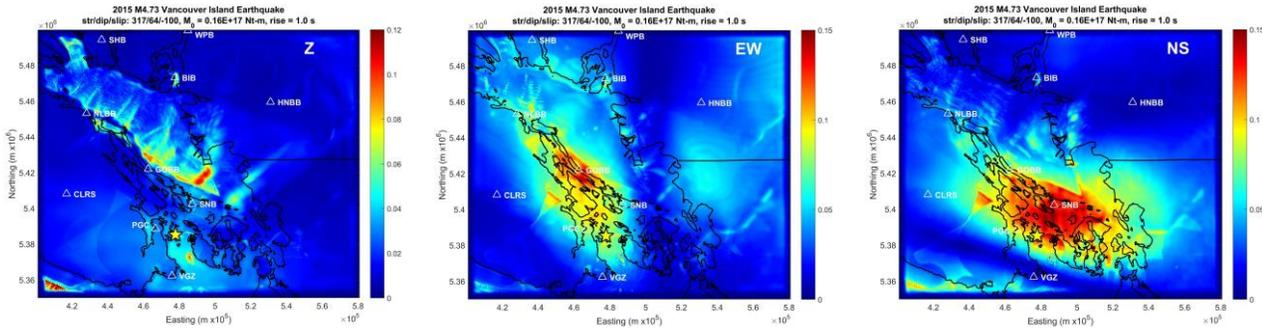
Figure 7. Predicted PGV maps of  $M 4.7$  Vancouver Island earthquake for Georgia basin region. Earthquake epicenter is shown by star. White triangles denote locations of selected earthquake recording sites labelled with code names.
