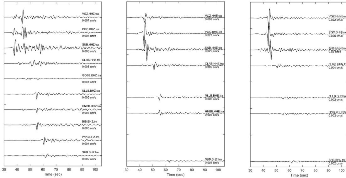
Figure 3. Broadband velocity time-series are low-pass filtered with a corner frequency of 0.5 Hz. Left panel shows the vertical components, and the middle and the right panels show the two horizontal (EW & NS, respectively) components.
